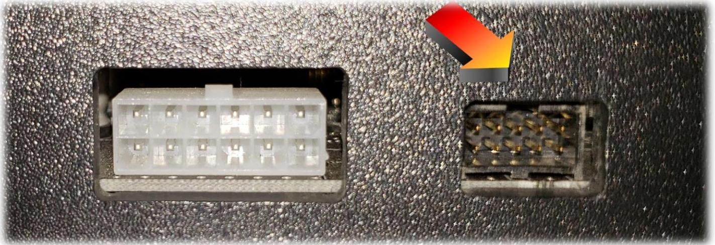
18. Then plug in the larger connector and make sure the clasp at the top locks and that both are firmly connected.
