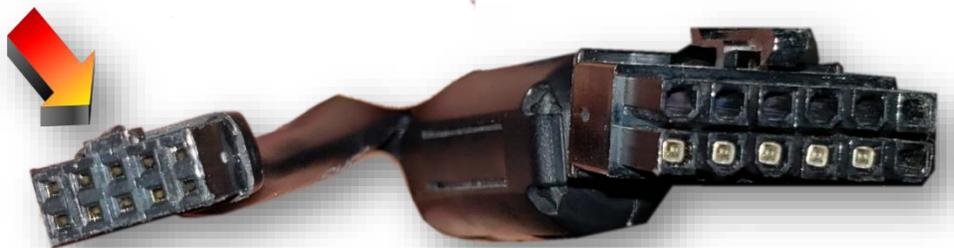
**!** WARNING: Please take note of the 10 gold pins on the smaller port. Incorrect installation of these connectors could create functionality issues. Be careful to properly insert them.
